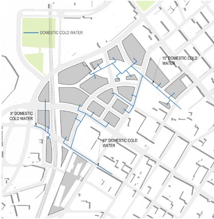
Proposed Domestic Water and Fire Protection Infrastructure
