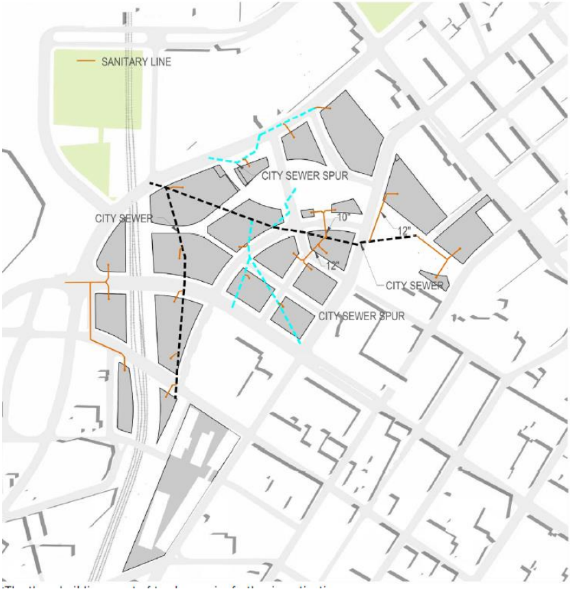
Proposed Sanitary Sewer Infrastructure
